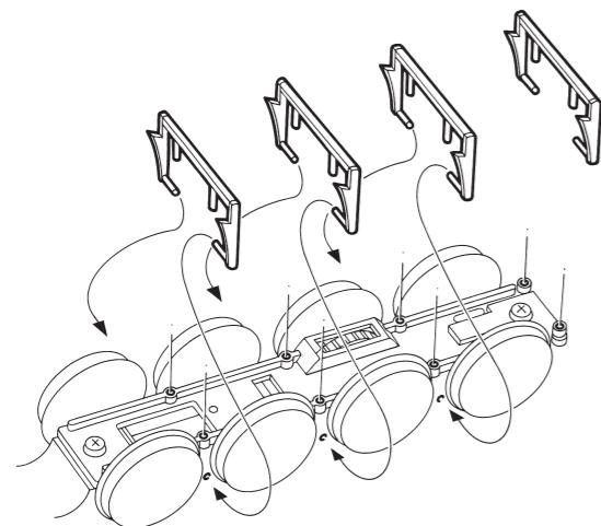
The Brake blocks in the enclosed bag can be mounted on the showcase model, as shown in the picture.
