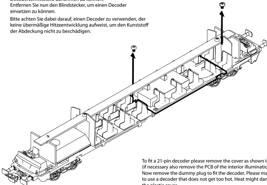
To fit a 21-pin decoder please remove the cover as shown in fig. 2 (if necessary also remove the PCB of the interior illumination).
